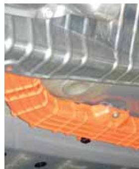
Electrical shield bolted to undercarriage
