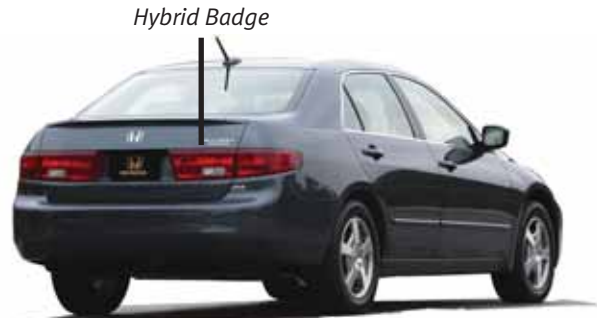
The word "Hybrid" appears directly under the name "Accord" above the right rear tail light.
