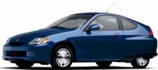
2000-2006 Insight models are 2-passenger cars with a distinctive aerodynamic shape and rear fender skirts.
