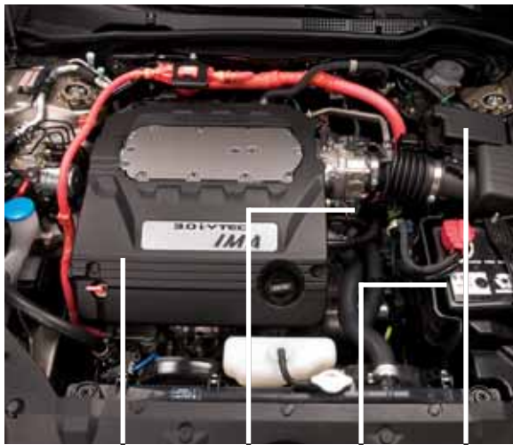
Engine Motor 12-Volt Battery Underhood Fuse Box
