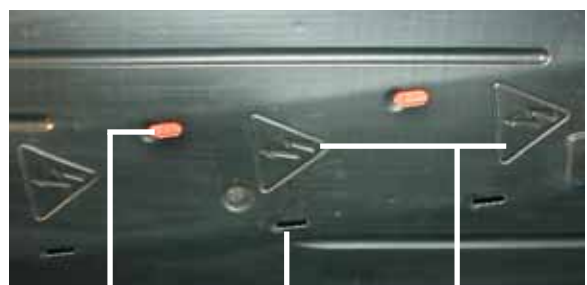
High-Voltage Cable Visible
