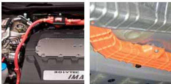
Orange cables under the hood, or orange shielding bolted to the undercarriage of a Honda tell you the vehicle is a hybrid.
