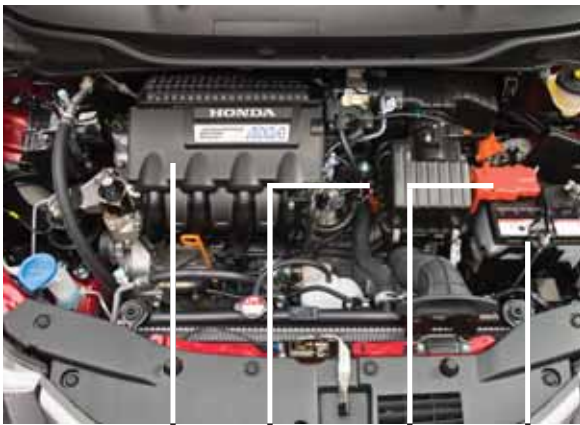
Engine Motor Positive Battery Terminal 12-Volt Battery
