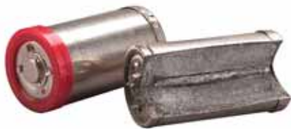
Electrolyte in the high-voltage battery cells is non-liquid and should not present a hazard.
